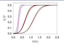
**Figure 3.**  $J_L/\gamma$  plotted against *V*, for T = 298 K,  $E_{AB} - \mu = 0.15$  eV, and a voltage sweep rate that for  $\gamma = 300$  s<sup>-1</sup> is u = 20 V/s. It is  $\lambda = 0$  (forward and backward sweeps in gray and pink, respectively),  $\lambda = 0.25$  eV (solid black and red lines), and  $\lambda = 0.5$  eV (black and red dashes). A small transient NDR is seen for  $\lambda = 0$  due to fast charge accumulation in the molecule, as given by dP/dt.<sup>41</sup>
